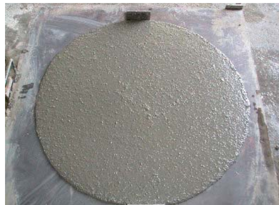
Photo 1 High strength fiber reinforced mortar
