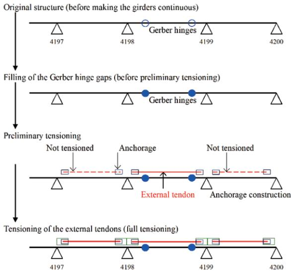
Figure-3 Steps to full tensioning
