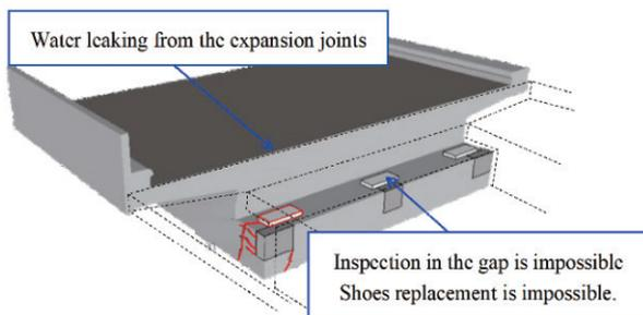
Figure-1 A Gerber hinge in a box girder
